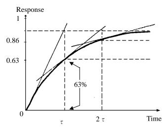
Figure 1.2 Response of a first-order measuring instrument
