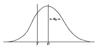
values obtained from the instrument **Figure 1.1 Distribution of data in instrument** under consideration. In this case, the following characteristics apply:
