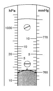
Figure 1.5 A vernier scale
