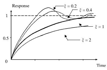
Figure 1.3 Response of a second-order measuring
